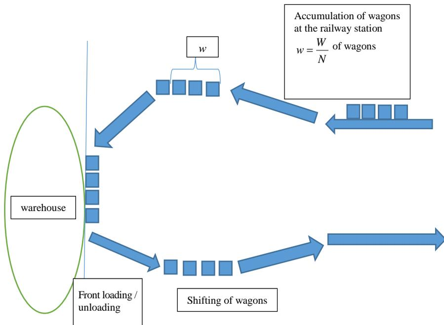
**Fig. 2.9.2. Scheme of accumulation of wagons at the railway station and supply / shift to / from the warehouse of the enterprise**
