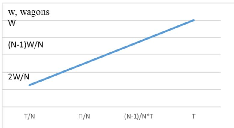
**Fig. 2.9.3. Scheme of accumulation of wagons for a time interval  $T$  ( $T = 24$  hours)**
