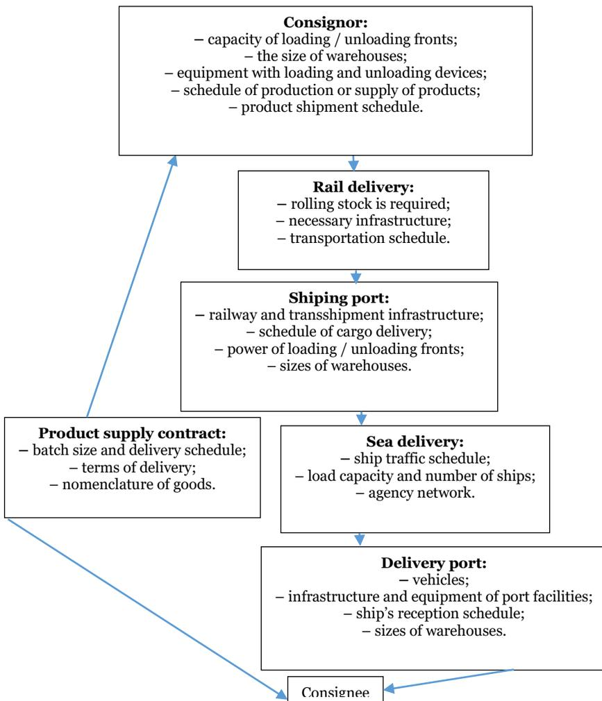
**Fig. 2.9.5. Structural block diagram of multimodal transportation by rail and sea**
